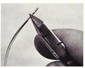
Photo 2. Clip off the wires, leaving about 1/8 inch of bare wire. When the wire is inserted into the connector, the insulation should be flush with the top of the connector pin.
